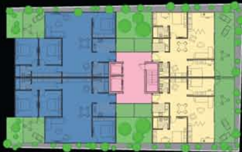
TYPICAL BLOCK 3 F5.1(BLUE) - F4.2(YELLOW) F5.1: FIVE-ROOM FLAT, 126 SQUARE METER F4.2: FOUR-ROOM FLAT WITH TERRACE, 100 SQUARE METER
