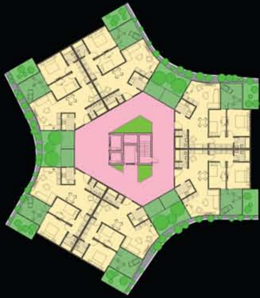
TYPICAL BLOCK 1 F4.3(YELLOW) - F4.3(YELLOW) - F4.3(YELLOW) F4.3: FOUR-ROOM FLAT AT THE TRIAL CORNER, 87 SQUARE METER
